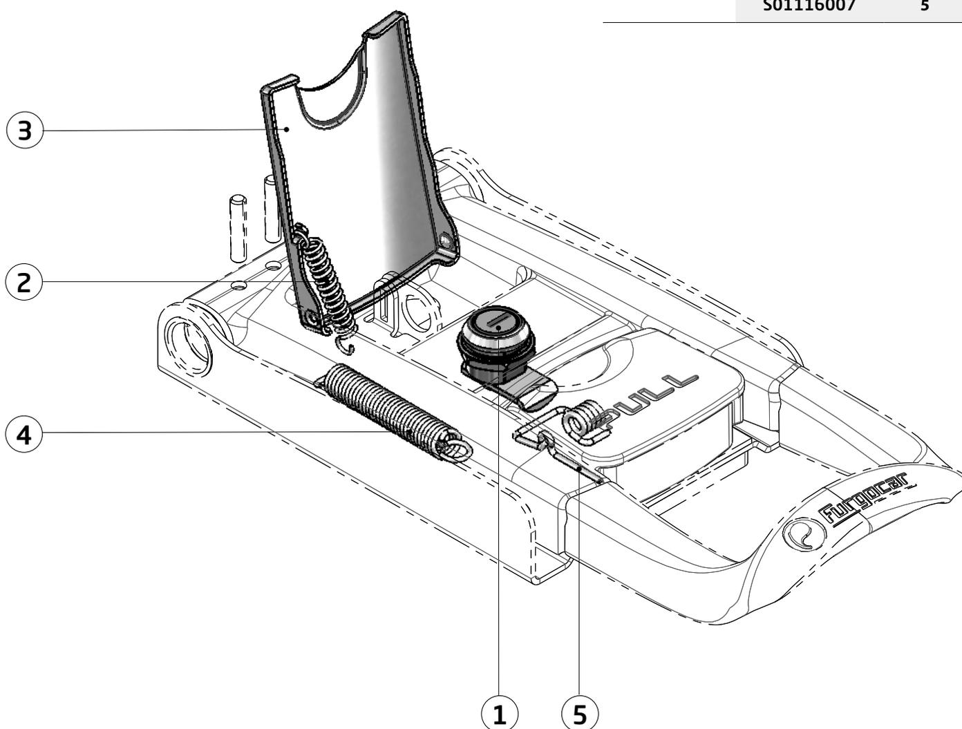
Poignées pour crémons en applique Ø16 inox / Handles for external locking gear Ø16 stainless steel
